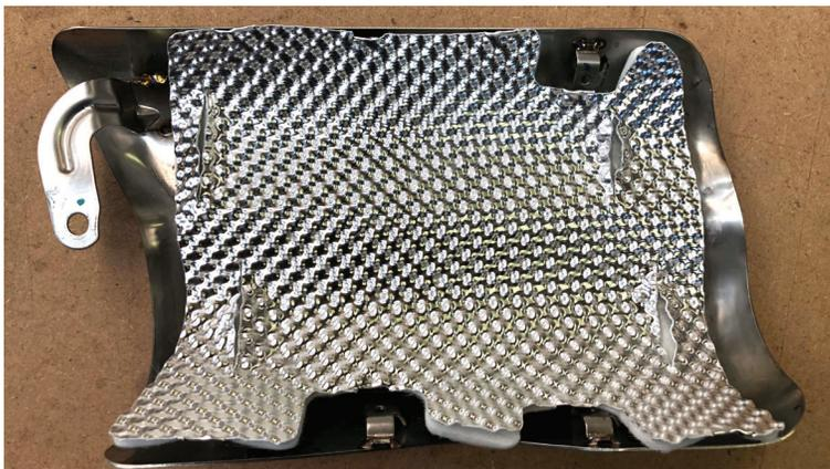
**FIG. 8** PRESS BACK INTO THE FACTORY STAINLESS SHIELD. THE SLITS WILL LINE UP AND YOU CAN BEND IT TO A SNUG FIT
