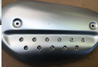
**STEP 3.** Take the rear aluminum factory shield and place the dimpled aluminum heat shield piece, on the inside of the factory shield, covering the holes. Cut 2 strips from the supplied reflective material (10x10 square material) to hold in place. FIG 2
