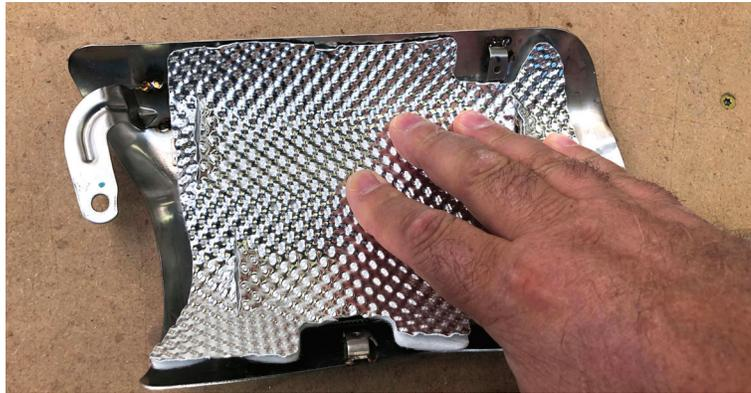
**FIG. 6** LAY GLASS FIBER IN CAT SHIELD THEN ALUMINUM SHIELD ON TOP AND PRESS DOWN AND FORM THE TWO PIECES TO THE CAT SHIELD.
